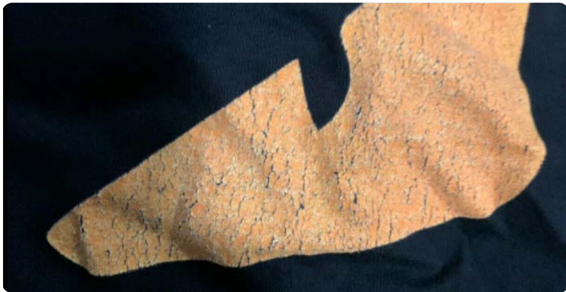
Cracks appearing after wash
